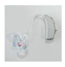
1. Disconnect the mould from the hearing aid where the tubing meets the sound hook. Hold the sound hook while pulling the tubing so as to not snap the hook. Turn/twist the tube to release it and then pull. Don't pull the tubing out of the earmould.
