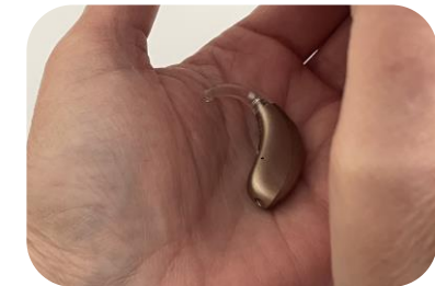
11. Check hearing aid is working in cupped hand. (you will hear a whistling noise)
