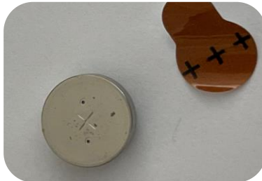
7. Make sure you have the right type of battery. Take the sticker off and wait for a few seconds.
