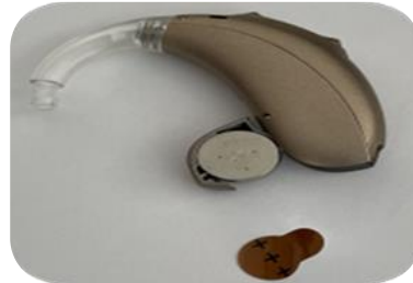
8. Insert battery with flat side up so you can see the cross. There is usually a picture in the battery compartment to help.
